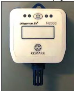
Figure 45. COMARK data logger N2003.
