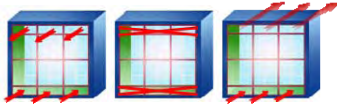
Figure 27. Operational modes of the DSF. External air curtain (left). Transparent insulation (centre). Preheating mode (right).
