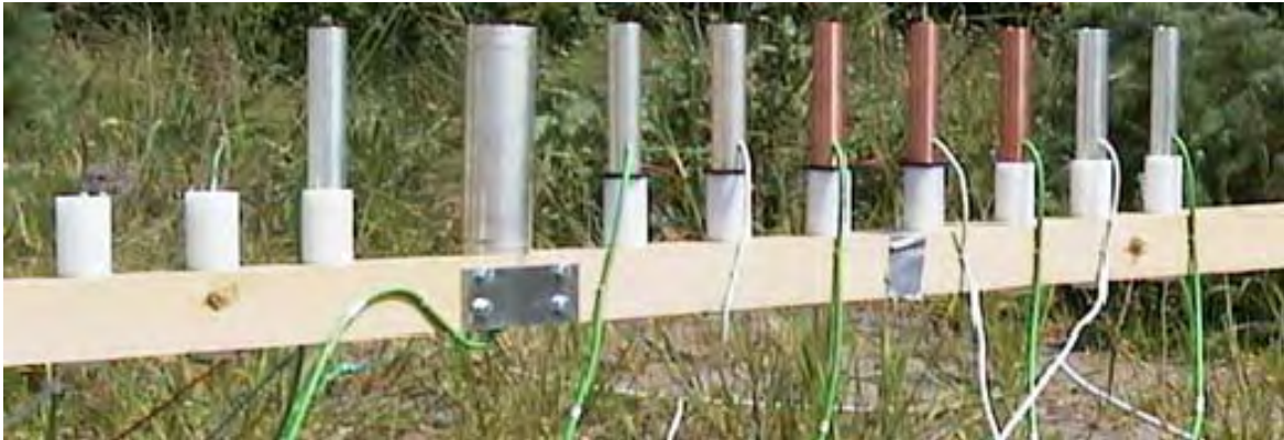
Figure 6. Experimental setup: testing of shielding techniques for air temperature measurements under direct solar access.
